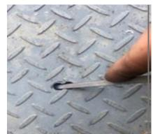
Open out the slots and dress to fit. Each Jackstrap may vary slightly so keep dressing and trial fitting until both sides accept both Jackstraps.
